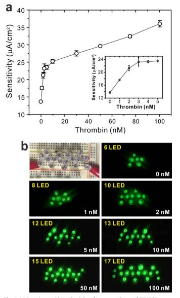
**Fig. 4.** (a) Detection sensitivity of anti-thrombin aptamer-decorated TENG biosensors depending on thrombin concentration. Inset graph shows the sensitivity after addition of thrombin in the low nanomolar range. (b) Photograph of the lighted LED lamp after interaction with various concentrations of thrombin.
