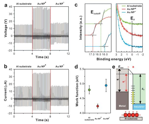
Fig. 2. (a, b) The output performance of Al-based TENGs with and without Au NP<sup>+</sup> or Au NP<sup>-</sup>. (c) UPS spectra and (d) work function of the reference Al layer, Au NP<sup>+</sup>-assembled and Au NP<sup>-</sup>-assembled TENG. (e) Energy band diagram of the Au NP<sup>+</sup>-assembled TENG. Yellow ovals and red circles indicate electrons and Au NPs, respectively. *w* and *w'* are work function and effective work function, respectively.
