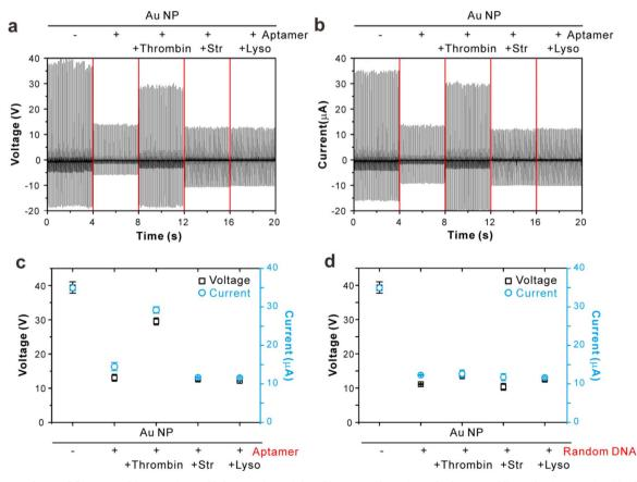
Fig. 3. (a) Output voltage and (b) current of the Au NP<sup>+</sup>-assembled TENG after anti-thrombin aptamer decoration and subsequent addition of various proteins. (c) Selectivity of anti-thrombin aptamer-decorated TENG biosensor for the detection of thrombin. (d) The output signals of random DNA-decorated TENG after addition of proteins.
